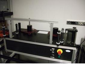
This is a fully loaded system with Kortho imprinter and custom sensor. These components are not normally included in quotes. The photos show the kind of customization possible with the GlueLogix Rewinder.
