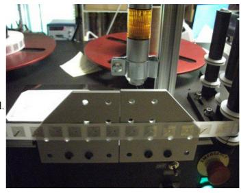
The rework surface is split to support razor splicing.
