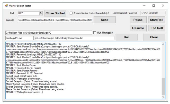
Start LineLogixPC from its installed shortcuts. Select an Operator and the provided test JOB file. Place a tag on the active antenna and watch prompts in LineLogixPC and Master Socket Tester. Allow access through your firewall if prompted. Click End Roll. Exit LineLogix.
