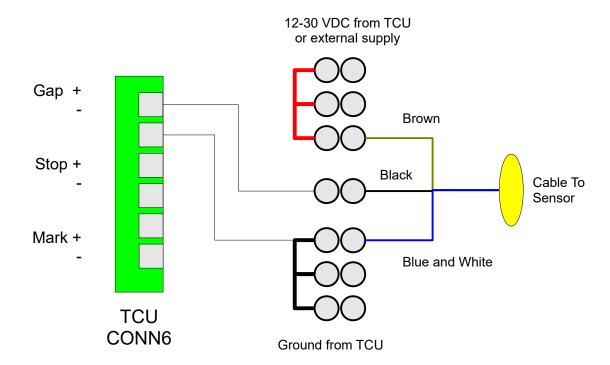
Other gap sensors can be integrated using the diagram above as a model. Be sure to select the correct Grayhill module to complete the input circuit.
