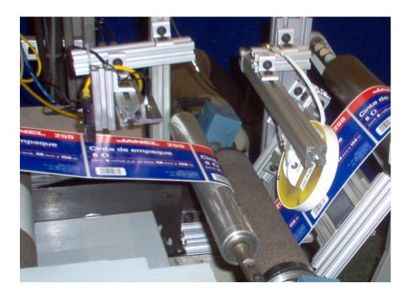
In this setup, paper moves to the right. The Gap Sensor (8) is on the left, just upstream of the first visible gap. The Gap Sensor had to be made movable with an elaborate 8020 bracket, because the antenna position was fixed by rollers. The sandwich configuration made up for reflections from rollers and other press components, made necessary by the tight spacing.
