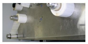
3. Assemble the gap sensor and antenna onto one piece of 80-20 to ensure alignment. Stand the assembly up on the table so that the web goes through the gap sensor and brushes the front of the antenna without deflecting:
