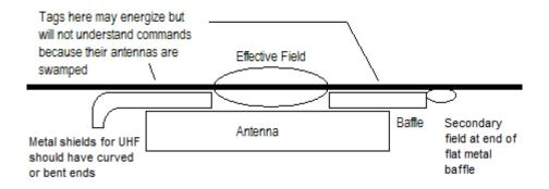
RFID tags MUST touch the shield material or be at most 1/16 inch away from the surface of the RF shields.
