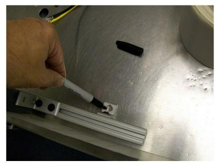
5. Drill pilot holes for wood screws that will grab the rewind table's wooden top under the steel shell:
