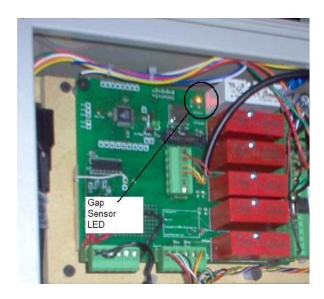
Slide the labels so that the gap is in the Gap Sensor.
